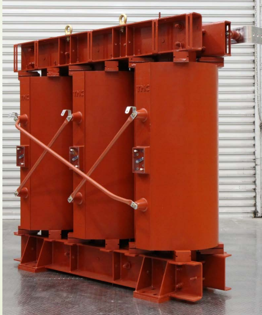
2000kVA 11000/433V Cast Resin Transformer, AN IP00
