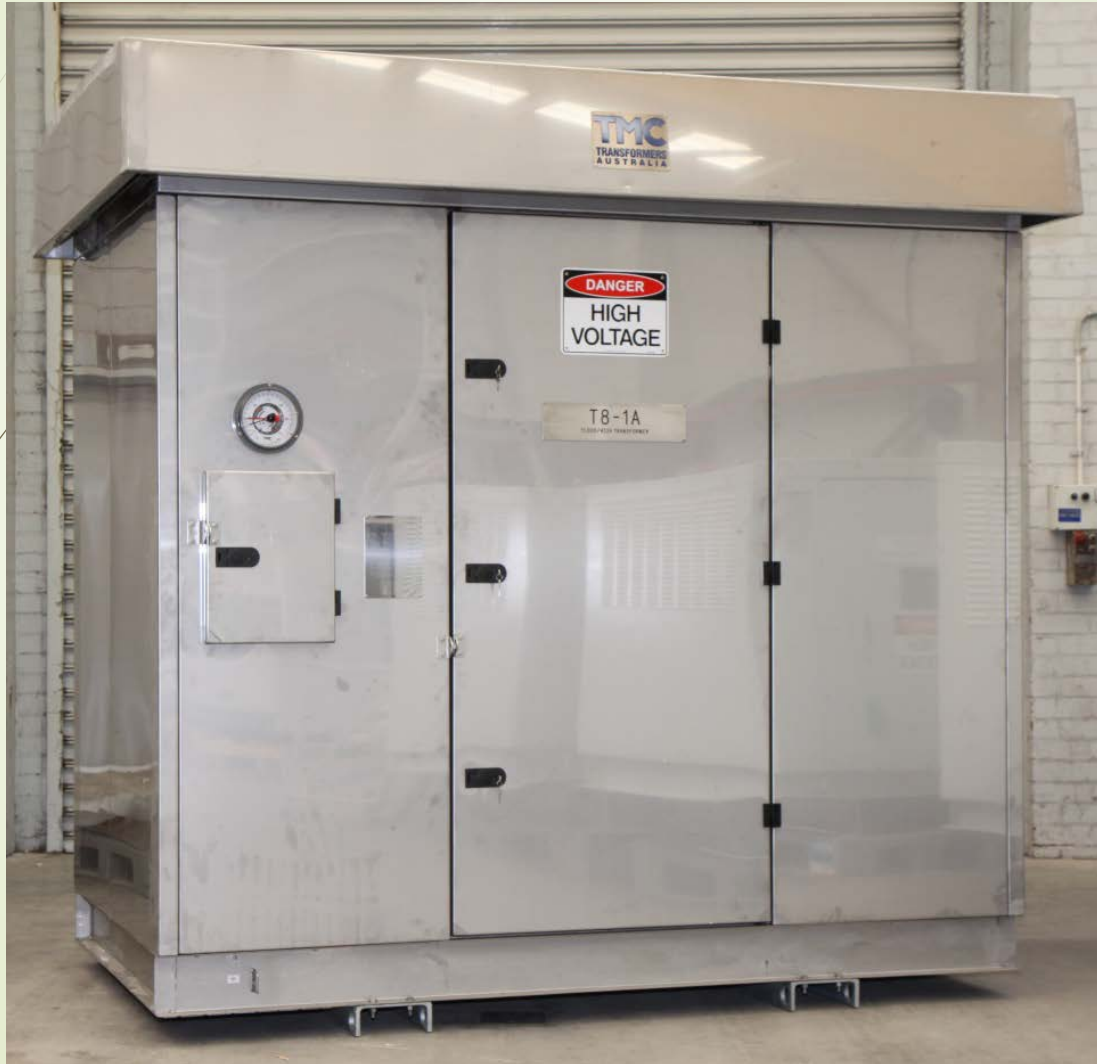
1500kVA 11000/433V Cast Resin Transformer, AN IP43 SS316
