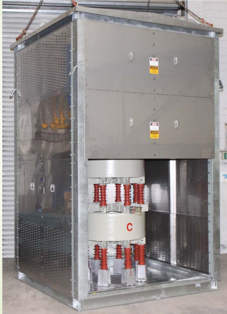
0.31mH 11kV 1312A Air Cored Current Limiting Reactor, AN IP43
