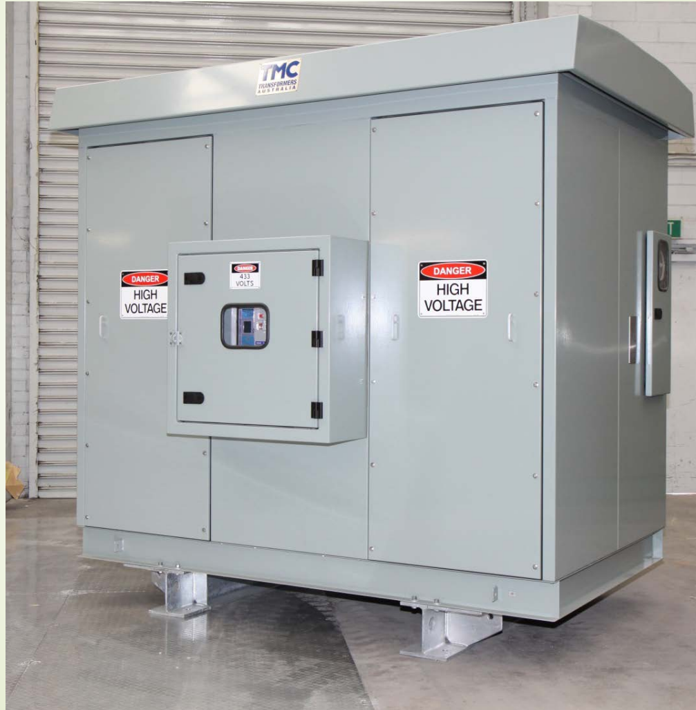
2000kVA 11000/433V Cast Resin Transformer, AN IP43 with MCCB on LV
