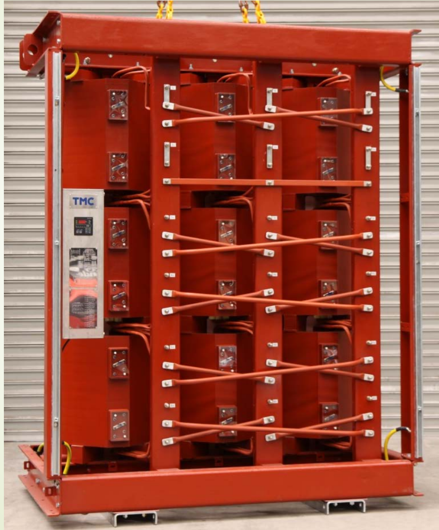
1750kVA 6600/1910V 36 Pulse Cast Resin Transformer, AN IP00
