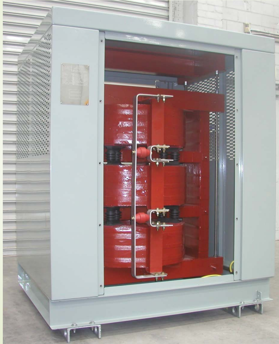
350kVAr 440V 459A Iron Shroud Reactor, AN IP21
